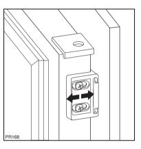
Fix cover (D) on guide (B) until it clips into place.
